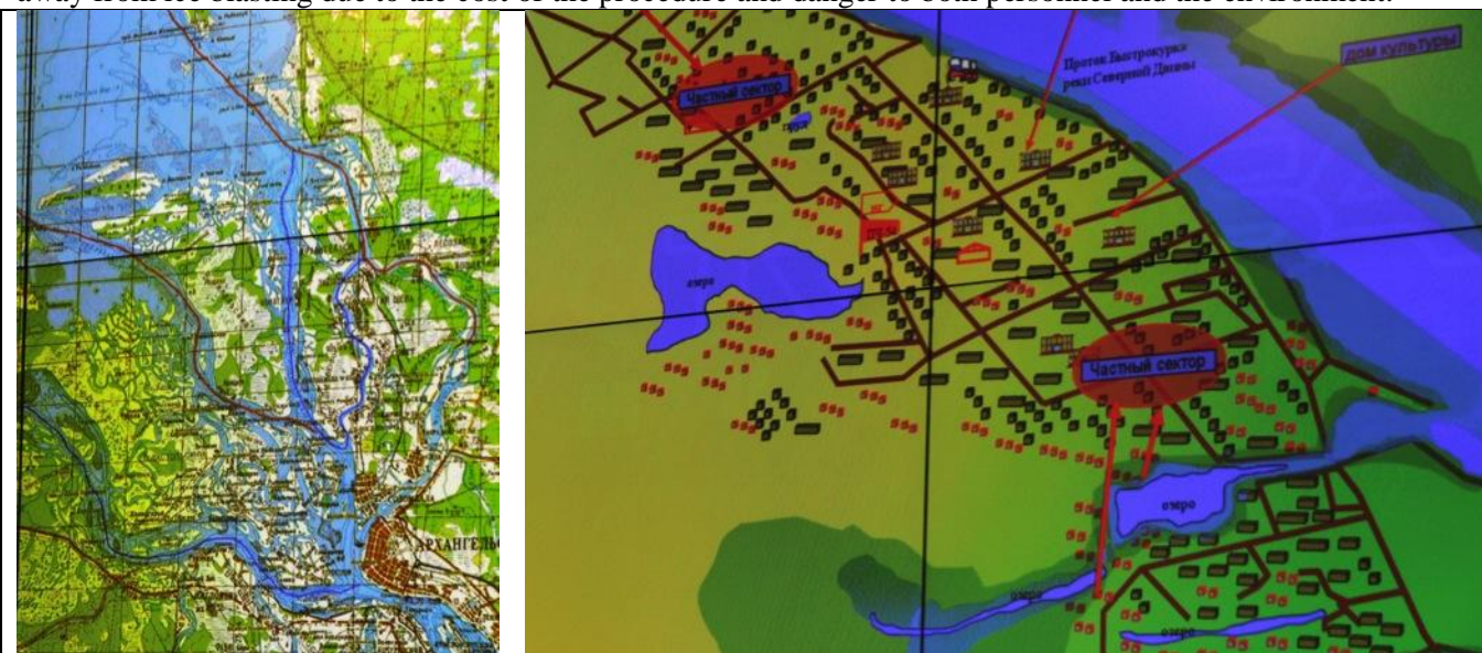
L: Preparing for mitigating breakup on the Dvina Delta, Arkhangelsk. Red lines denote paths for icebreakers to break ice; blues are for river ice that must be cut. R: Inundation model for town up-river....jce
