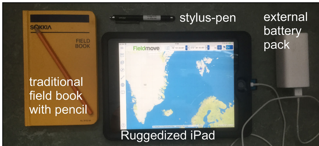
Figure 1. The digital field notebook used at UNIS. Hardware consists of a field-proofed iPad 9.7". An external battery pack that can be kept in an inside pocket is essential during winter-spring field work. The stylus-pen significantly improves usability in cold and windy conditions.
